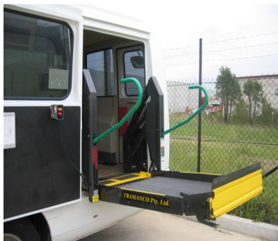
Side Loading Hoist
